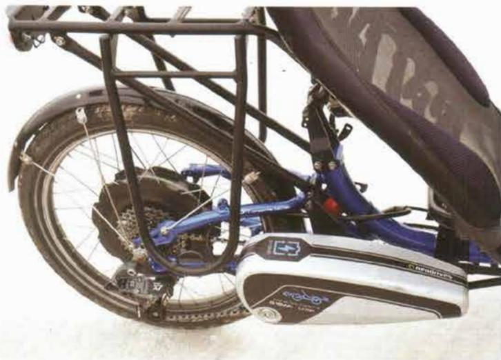
**LEFT:** Battery is mounted as low as possible and out of harm's way. A second battery can also be added. Removal is a one-key operation, but charging is possible in-situ.
